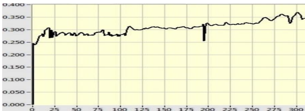
Fig. 7: variation of friction coefficient with time at 450°C in AISI H11 (Sample1) specimen
