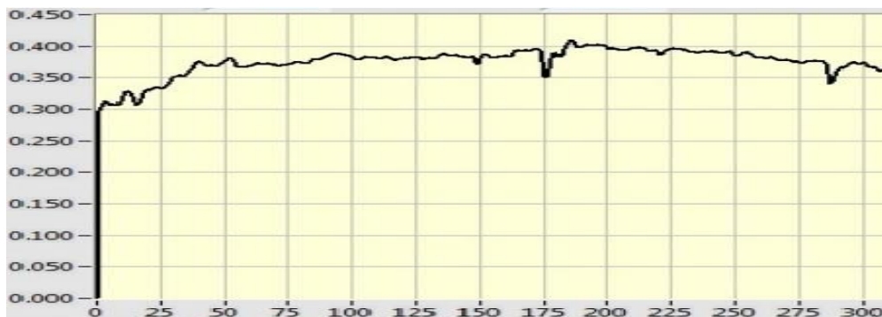
Fig.6: variation of friction coefficient with time at 450°C in AISI L6 (Sample1) specimen
