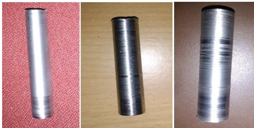
Fig.2: Test specimens of AISI L6, AISI H11 and AISI O1.
